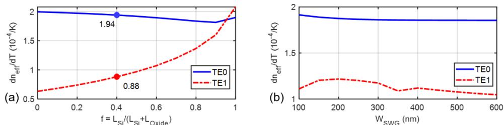
Fig. 2. (a) Thermo-optic coefficient versus duty ratio for a mode sensitive TOPS with  $W_{\text{SWG}} = 500 \text{ nm}$ . (b) Thermo-optic coefficient versus  $W_{\text{SWG}}$  for  $f = 0.7$ .
