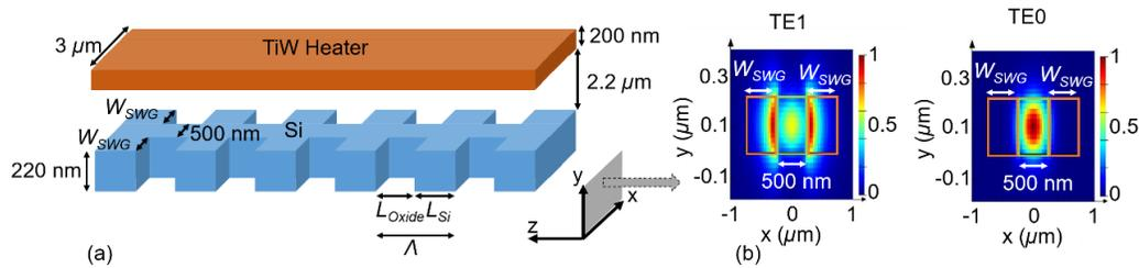
Fig. 1. (a) Schematic view of SWG-based mode-sensitive TOPS, (b) Normalized electric field distribution for TE0 and TE1 ( $f = 0.7$  and  $W_{\text{SWG}} = 500 \text{ nm}$ ).
